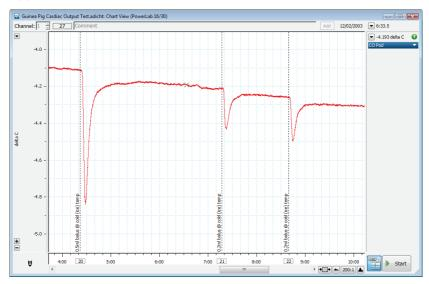
Guinea pig cardiac output determined by the thermodilution method. Bolus of cold saline is injected into the jugular vein and temperature probe is placed in the carotid artery.
