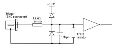
In the contact closure mode, the trigger input will respond to a direct short between the center pin and outer ring of the BNC. This can be achieved with an external relay contact, push-button or microswitch. The trigger input is not isolated when set up for contact closure.
