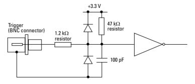
In order for the external trigger to work, a voltage must be applied between the outer ring and the inner pin of the connector. Applying a voltage just to the center pin may not work. The source must be capable of supplying at least  $100 \, \mu A$  of current to activate the trigger.
