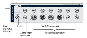
The front panel of the PowerLab 16/35 is also similar to the other two PowerLabs except it has sixteen BNC connectors (marked Input 1-16) with four alternative pod (DIN) connectors for Inputs 1-4, for recording external signals.
