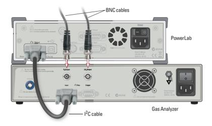
Use two BNC cables to connect the  $CO_2$  and  $O_2$  analog outputs on the back panel (Figure 2–1) of the Gas Analyzer to two available inputs on the front panel of your PowerLab. Any free inputs on the PowerLab can be used for other measurements.
