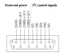
Figure A–10 The pin assignments for the  $I^2C$  port G
