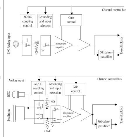
The input amplifiers can be set to pass both DC and AC signals, or to pass only AC signals without passing DC signals. Input impedance is one megohm (1  $M\Omega$ ).
