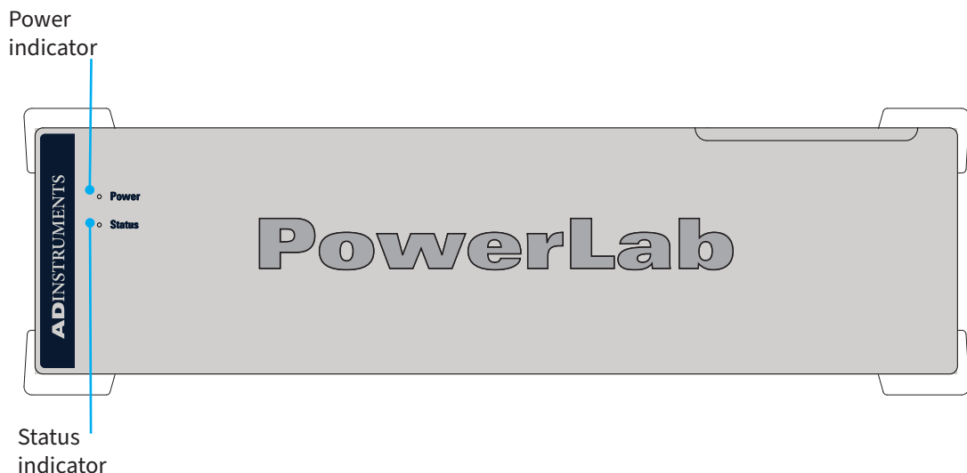
Figure 4–2 The front panel of the PowerLab C
