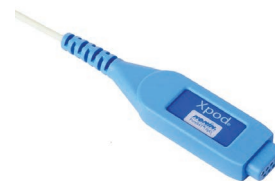
Wired SpO 2 Adapter. Connects the MLT321 SpO 2 Finger Clip to an Equivital Belt.
